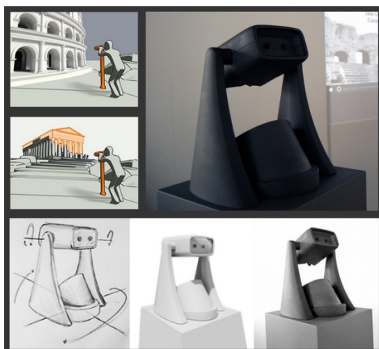
Figure 11: DIVAR. Below sketch, 3D Model and Device Made (photo and SpinVector processing)
