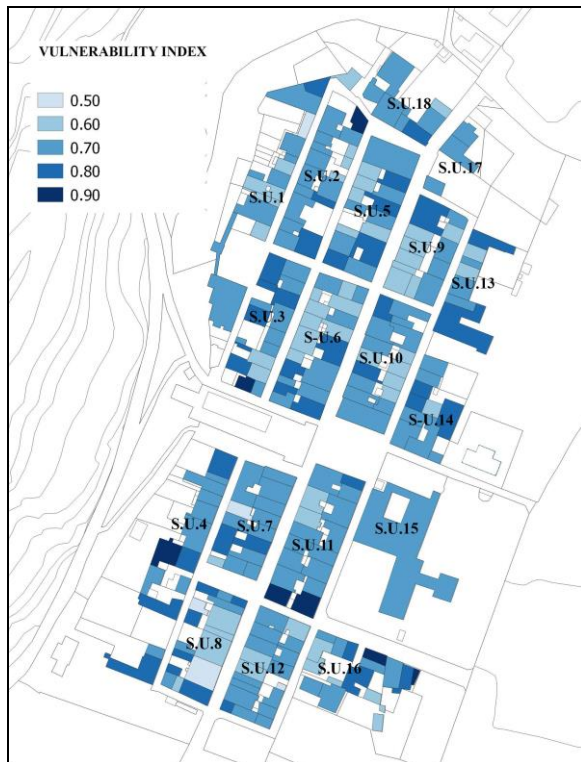
Figure 3. Macroseismic Vulnerability Index of a part of the city of Scarperia. The results are extracted from the GIS platform.
