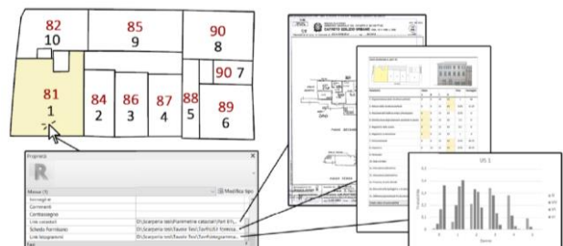
Figure 8. Digital information provided into the H-BIM at AL (Bonaguidi, 2019).
