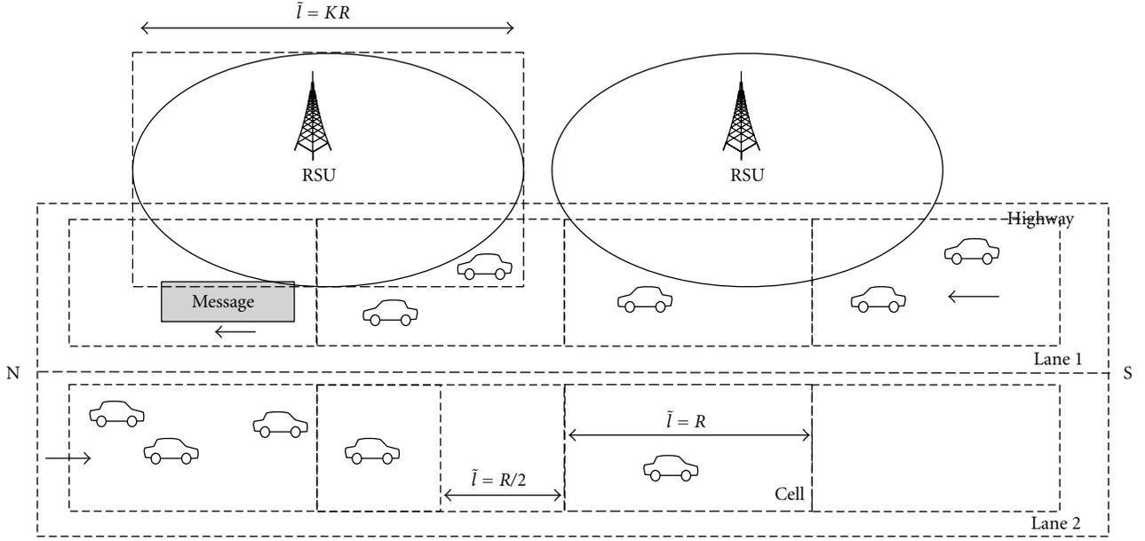
FIGURE 3: Vehicular grid comprised of  $\tilde{l}$ -size RSU virtual and wireless V2V cells. The probability that a vehicle is connected via V2V and V2I depends on the cells occupancy.
