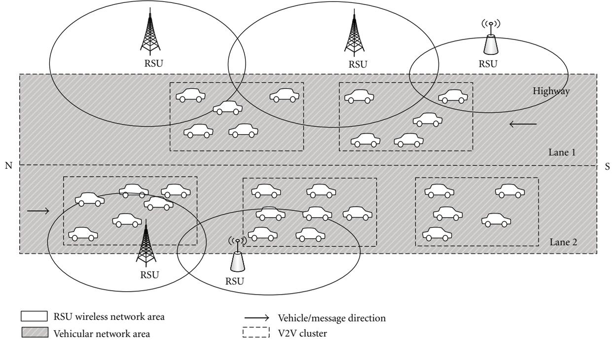
FIGURE 1: Vehicular grid with an overlapping heterogeneous wireless network infrastructure.
