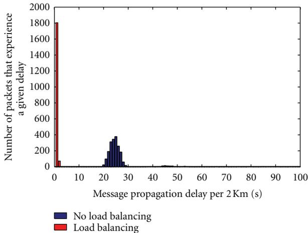
FIGURE 12: Number of packets experiencing different message propagation delays at the vehicle density of 65 [veh/km] and HP message probability of 0.4.
