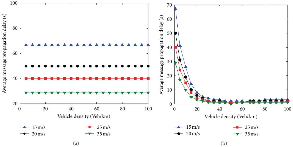
FIGURE 5: (a) Average message propagation delay for increasing vehicle density, and speed for Phase 1 (no connectivity) at different speeds (i.e., 15, 20, 25, and 35 m/s). (b) Average message propagation delay for increasing the vehicle density at different traffic speeds using V2V communication.
