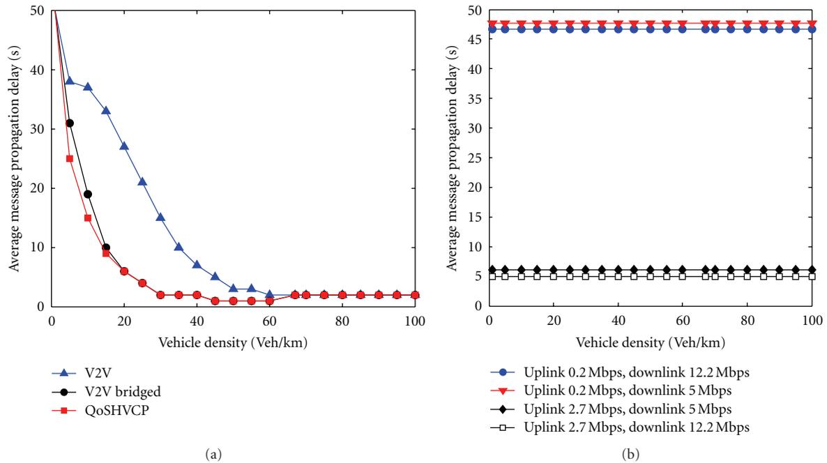
FIGURE 6: (a) Average message propagation delay for increasing vehicle density for V2V, V2V bridged and QoS HVCP at fixed speed. (b) Average message propagation delay for increasing vehicle density in V2I communications at different uplink and downlink rates.
