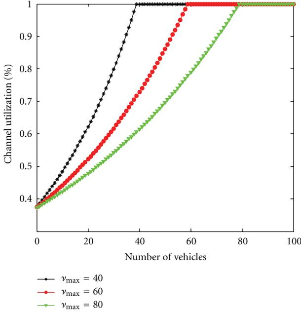
FIGURE 2: Percentage of *channel utilization* in an RSU wireless network for HP messages delivery, with  $\nu_{\max} = [40, 60, 80]$ .
