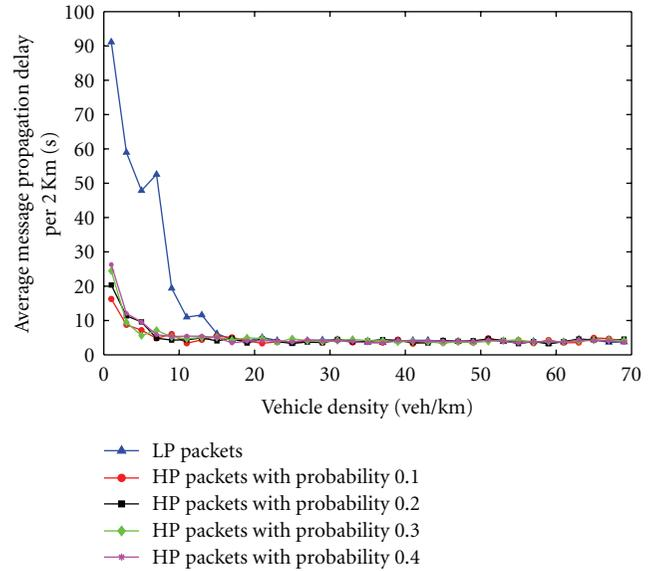
FIGURE 9: Message propagation delay for high and low priority messages with different HP probabilities with load-balancing mechanism.
