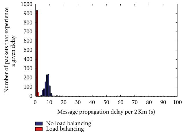
FIGURE 10: Number of packets experiencing different message propagation delays at the vehicle density of 65 [veh/km] and HP message probability of 0.2.
