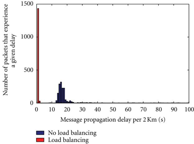
FIGURE 11: Number of packets experiencing different message propagation delays at the vehicle density of 65 [veh/km] and HP message probability of 0.3.
