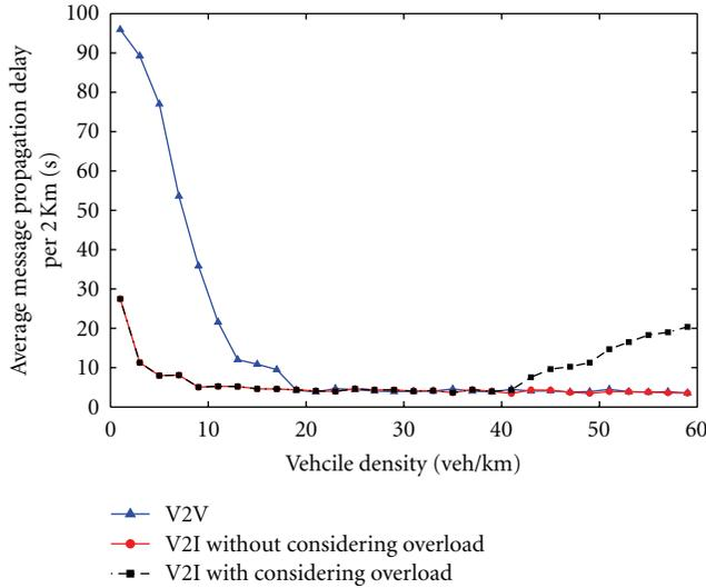
FIGURE 7: The effect of the network overload on both V2V and V2I, versus the vehicle density.
