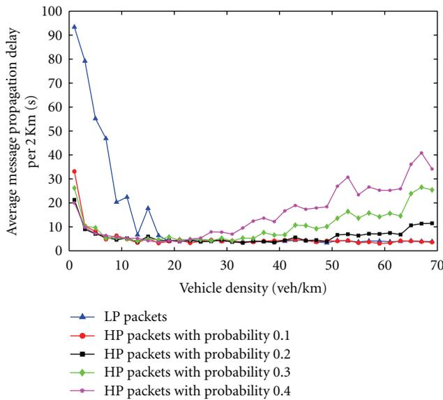
FIGURE 8: Message propagation delay for high and low priority messages with different HP probabilities without load-balancing mechanism.
