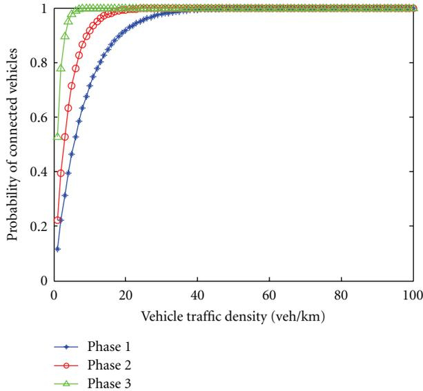
FIGURE 4: Probability of connected vehicles in Phases 1–3 versus the vehicle traffic density.
