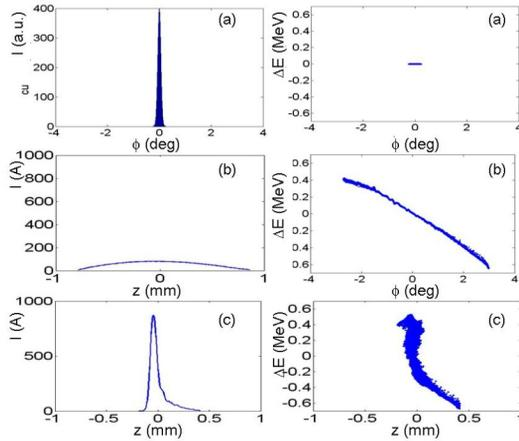
Fig. 2. Bunch (a) at cathode, (b) at exit of linac and (c) at the exit of the compressor. Left and right frames, respectively: longitudinal profile and  $\Delta E(\text{MeV})$  vs length.
