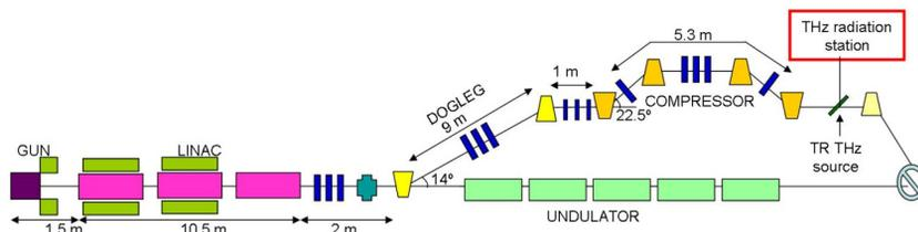
Fig. 1. Cartoon of the SPARC photoinjector with a THz radiation station downstream a dogleg and compressor, where bending and quadrupole magnets are marked by yellow wedges and blue lenses, respectively.
