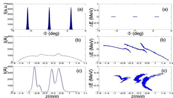
Fig. 5 Three pulses comb beam (a) at cathode; (b) at exit of linac and (c) at the exit of the magnetic compressor ( $R_{56} = -120 \text{ mm}$ ). Left and right frames: longitudinal profile and  $\Delta E(\text{MeV})$  versus length, respectively.
