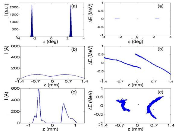
Fig. 4. Two pulses comb beam (a) at cathode; (b) at exit of linac and (c) at the exit of the magnetic compressor ( $R_{56} = -100$  mm). Left and right frames: longitudinal profile and  $\Delta E(\text{MeV})$  versus length, respectively.
