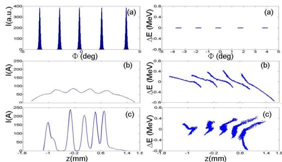
Fig. 6 Five micro-pulses comb beam (a) at cathode; (b) at exit of linac and (c) at the exit of the magnetic compressor ( $R_{56} = -120 \text{ mm}$ ). Left and right frames: longitudinal profile and  $\Delta E(\text{MeV})$  versus length, respectively.
