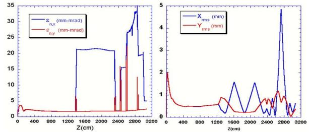
Fig. 3 Left and right frames, respectively show the beam emittance and envelope evolution for the single pulse case from cathode to the magnetic compressor exit
