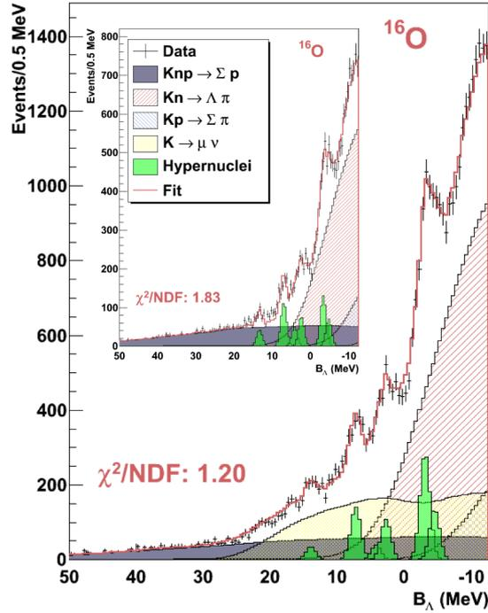
**Figure 3.** Excitation energy spectrum of  $^{16}_{\Lambda}\text{O}$  obtained with the  $(K_{\text{stop}}^-, \pi^-)$  reaction by the FINUDA experiment (from [91]). The inset shows the binding energy distribution for a data sample free from the background due to  $K^-$  in flight decay.
