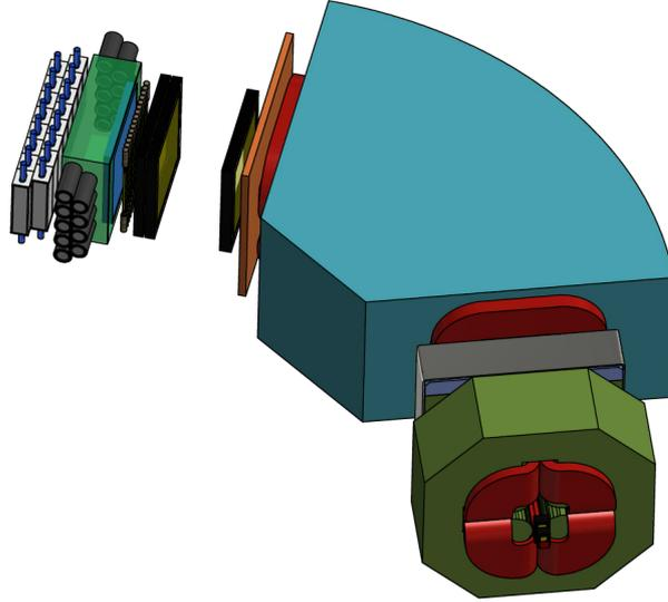
**Figure 10.** Schematic view of the  $S$ - $2S$  spectrometer for the  $(K^-, K^+)$  reaction. It consists of three magnets  $QQD$  (two quadrupole magnets and one dipole magnet).
