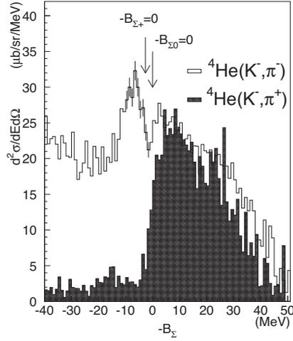
**Figure 6.** Excitation energy spectra of  ${}^4\text{He}(K^-, \pi^-)$  and  ${}^4\text{He}(K^-, \pi^+)$  at 600 MeV/ $c$   $K^-$  momentum, measured at  $4^\circ$  (from [212]).
