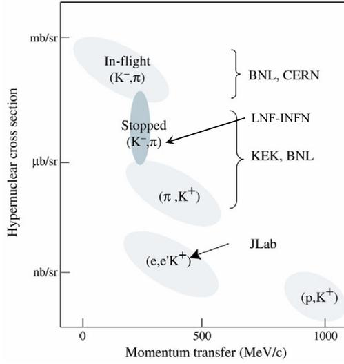
**Figure 2.** Cross section for typical hypernuclear production reaction as a function of the transferred momentum (adapted from [10]).
