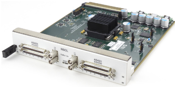
Fig. 5. Photograph of the CoBo. The front panel consists of 4 VHDCl connectors to connect up to 4 AsAd cards, 4 configurable LEMO connectors, and a micro-USB interface for monitoring. The CoBo conforms to the MicroTCA.0 R1.0 PICMG double-width full-height standard.
