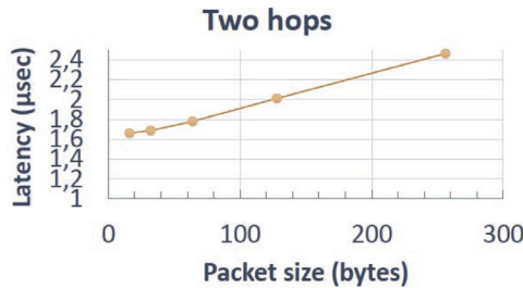
Fig. 8. One-way packet latency versus packet size for a double hop configuration.
