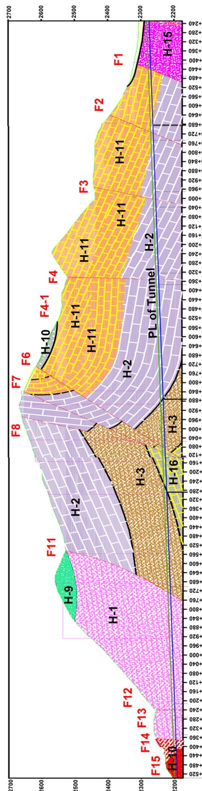
Fig. 1 The route of Tunnel in different formations [35]
