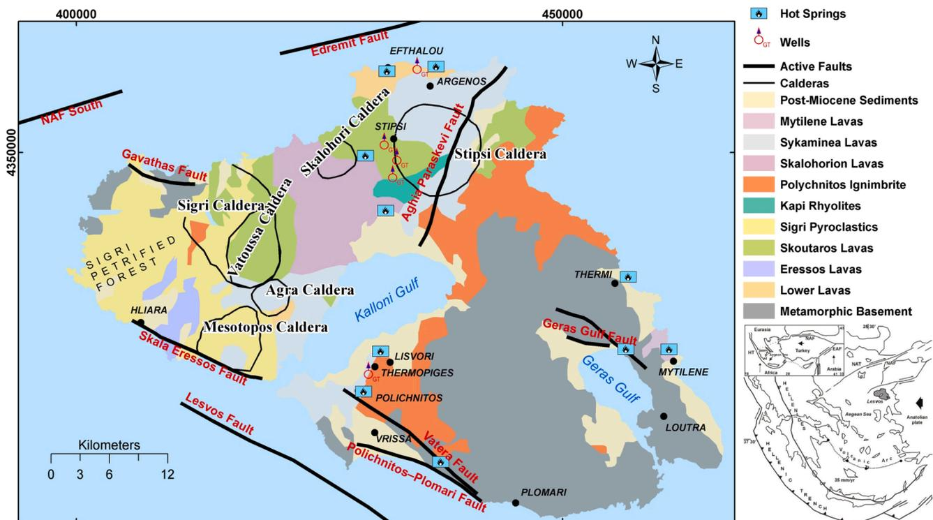
Fig. 1. Location map of Lesvos island with overlay of the caldera structures (adopted from Kouli and St. Seymour, 2006), hot springs and wells locations (after Mendrinou et al., 2010) and major active faults (adopted from Ganas et al., 2013). Inset: Map presenting the general geodynamic context in the eastern Mediterranean Sea. NAF: Northern Anatolian Fault, NAT: Northern Aegean Trough (modified from McKenzie, 1972).
