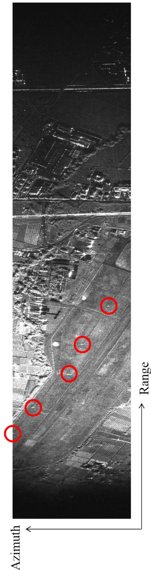
**Fig. 4.** Multi-look amplitude SAR image of a  $0.55 \text{ km} \times 2.8 \text{ km}$  wide patch of the entire acquired strip. Spatial resolution:  $1.5 \text{ m (range)} \times 1.25 \text{ m (azimuth)}$ . Red circles indicate the CRs' positions. (For interpretation of the references to colour in this figure legend, the reader is referred to the web version of this article.)
