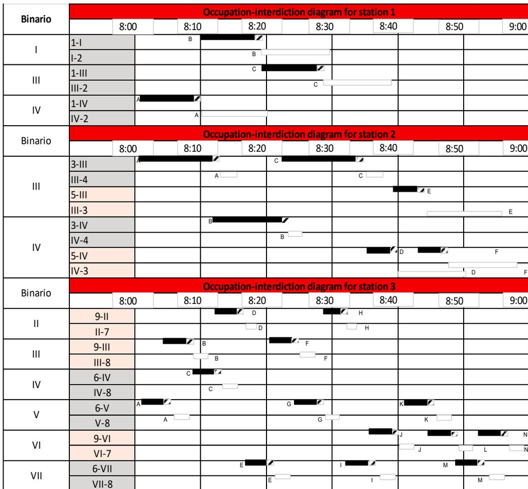
Fig. 6. Occupation-interdiction diagrams for stations 1, 2 and 3
